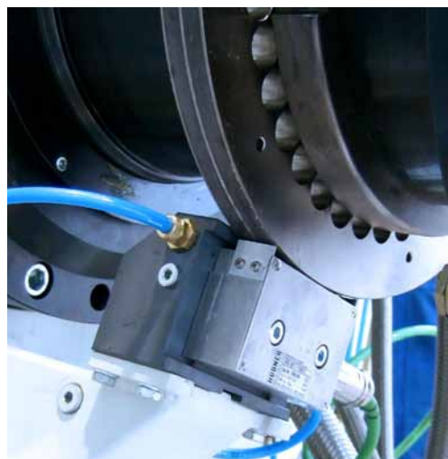
The magnetic hollow shaft encoders HDmag with an inside diameter of up to 740 mm can be installed directly on the engine hub.
